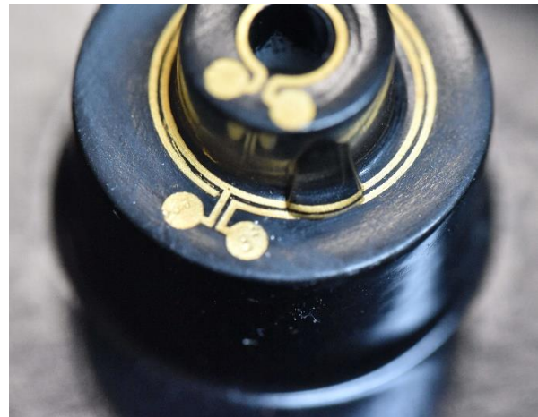
Two parallel printed conductive paths facilitate resistive moisture measurement
